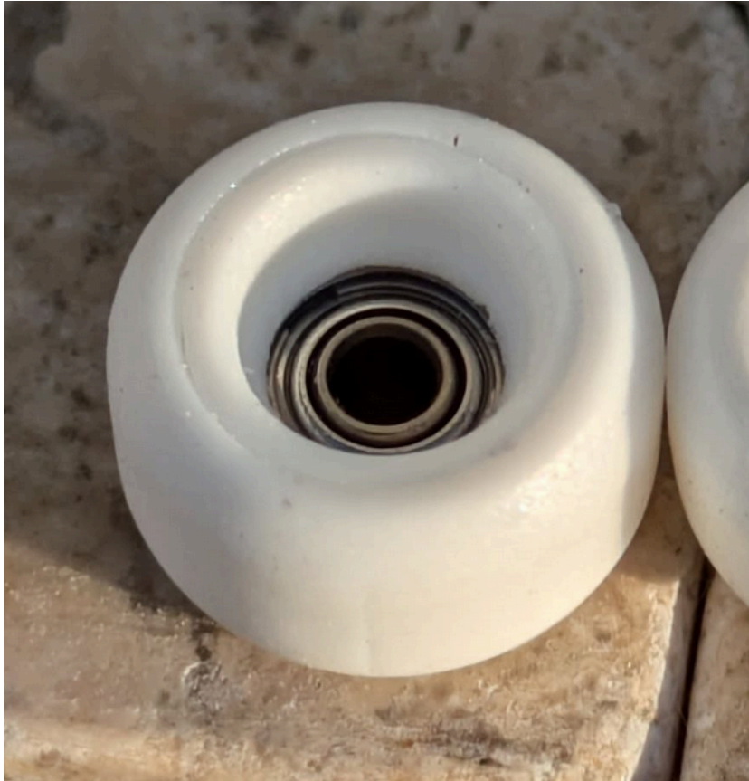
Finished wheel, with the bearing properly secured by the ring.
